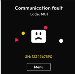
A screenshot of a Nayax device screen showing a communication fault. The text "Communication fault" and "Code: M01" are at the top. Below is a sad face icon. The text "SN: 1234567890" and "Menu" are at the bottom.                                                  | Verify network settings in the Device information (menu) or Nayax Core. Ensure the Ethernet, Wi-Fi, or SIM connection is stable. |
